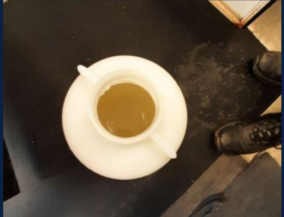
Final discharge with persistent foam/scum/solids, final effluent sample with amber color.
